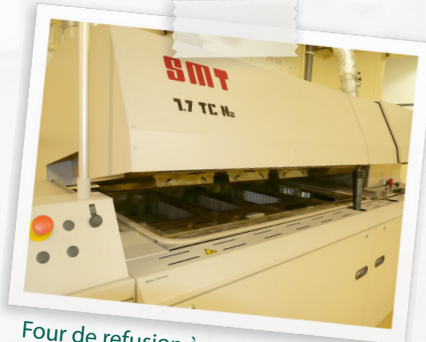
Four de refusion à convection forcée 4 zones SMT 1,7TC N2
